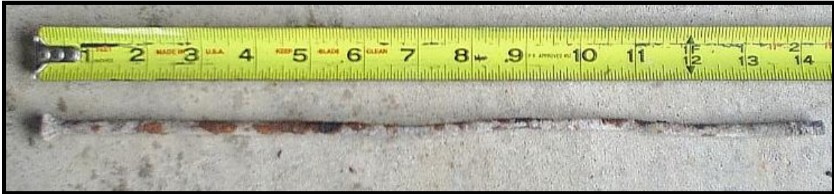
14-inch threaded bolt for box buggy seat
