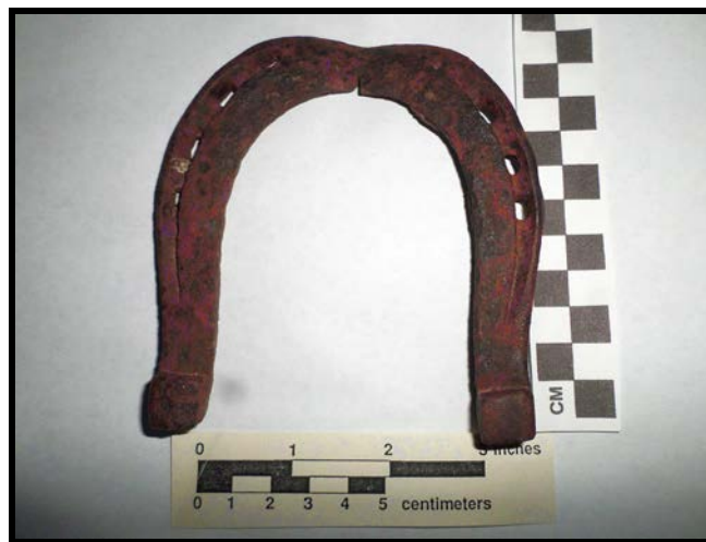
Hand-forged Spanish Mule shoe with crack and heavy wear
