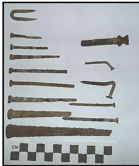
Assorted nails, staple (left) square nails (right) round/wire nails
