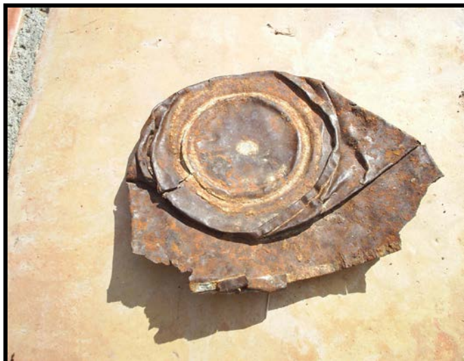
Lead-soldered lap side seam No.2 can
