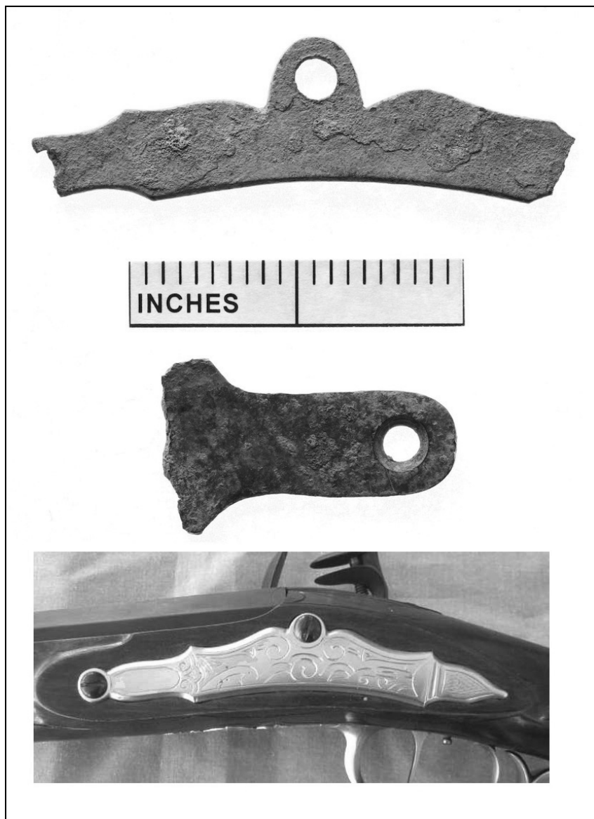
Figure 3.3: Firearm sideplate fragments (top and middle), Fort Pierre Chouteau. Below—sideplate, reproduction flintlock (from www.whitemuzzleloading.com/archives.htm ).
