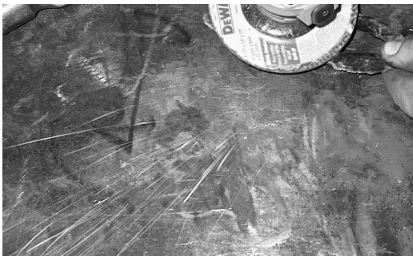
Figure 5.3: Result of spark test on wrought iron chain link.
