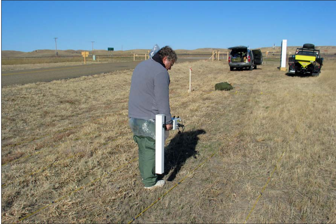
Figure 13. Conducting the magnetic survey with a Geoscan Research FM36 fluxgate gradiometer in Grid Area 7 (view to the north northwest).
