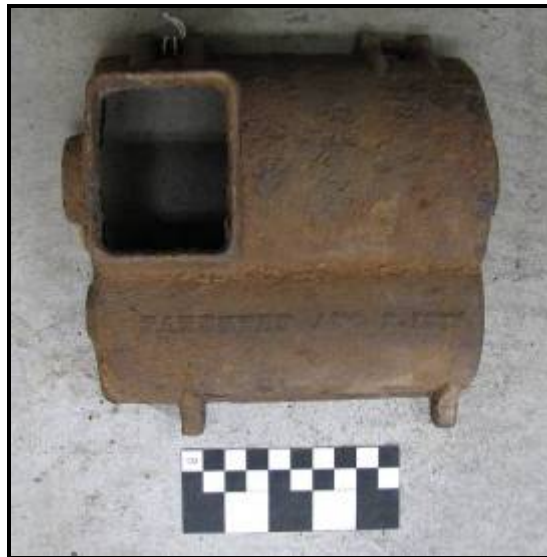
Figure 5-68: Machine cover from harness machine (catalog #2137) with patent date August 2, 1839. Photo by author.
