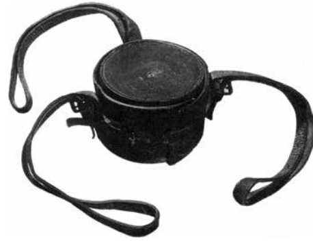
LEFT A brass pendulum odometer fits inside the brass case at right. The case, in turn, is placed inside the frame. The whole assembly is then inserted into the leather carrier (ABOVE) and strapped to the spokes of the wagon wheel. HENRY FORD MUSEUM & GREENFIELD VILLAGE, DEARBORN, MICHIGAN.
