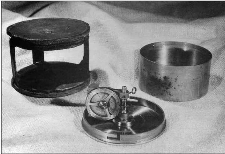
LEFT A brass pendulum odometer fits inside the brass case at right. The case, in turn, is placed inside the frame. The whole assembly is then inserted into the leather carrier (ABOVE) and strapped to the spokes of the wagon wheel. HENRY FORD MUSEUM & GREENFIELD VILLAGE, DEARBORN, MICHIGAN.
