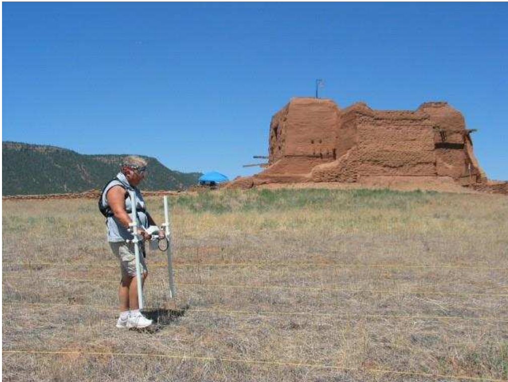
Figure 14. Conducting the magnetic survey with the dual fluxgate gradiometer (view to the west southwest)
