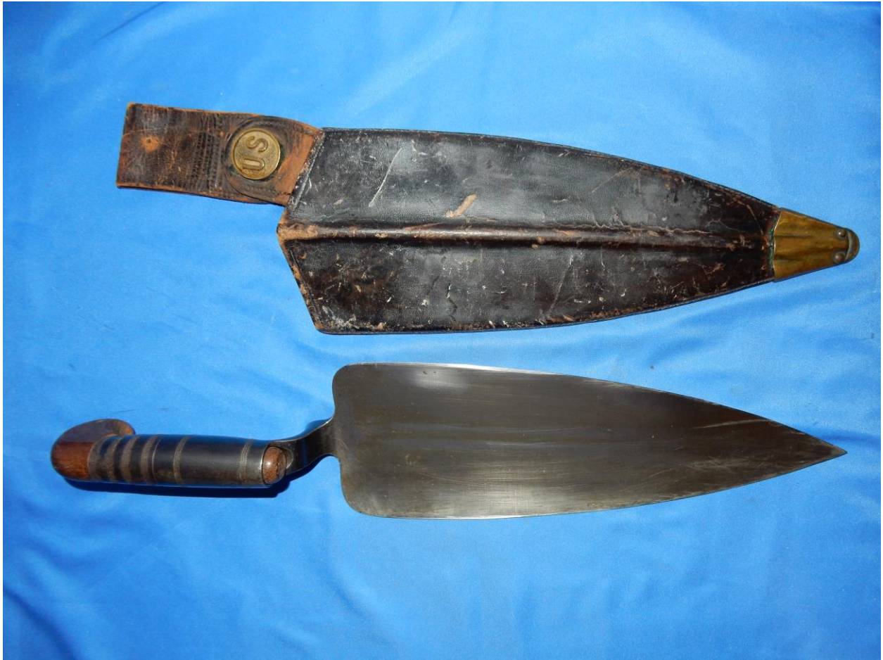
Figure 16. The trowel bayonet developed by Edmund Rice. During field trials it saw actual combat use at the Big Hole Battle in 1877. As a bayonet it was a failure, but as an entrenching tool it worked well. Author's collection.
