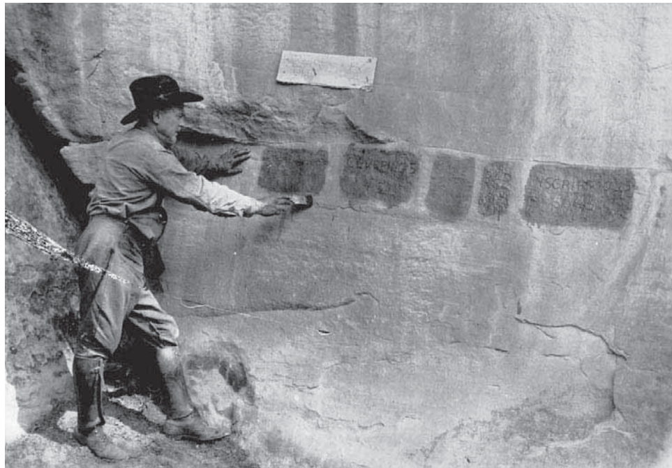
Figure 4.4: Off the main trail, Vogt created an inscription that read “Colourless coverings save old inscriptions” to test various consolidants on the sandstone. Source: Vogt Photos, El Morro Archives, n.d.
