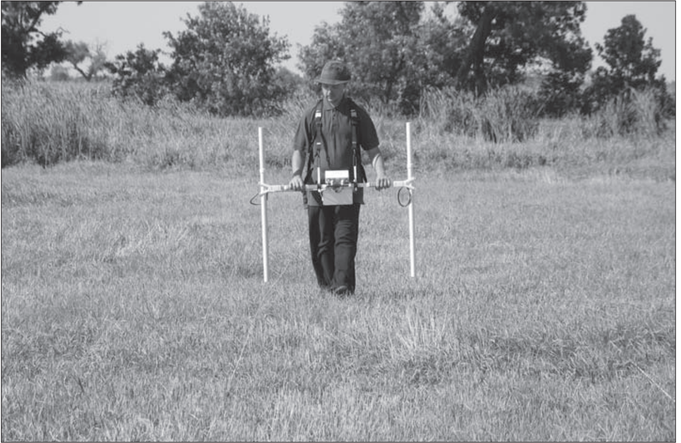
FIGURE 6. Conducting the magnetic survey with the dual fluxgate gradiometer.
