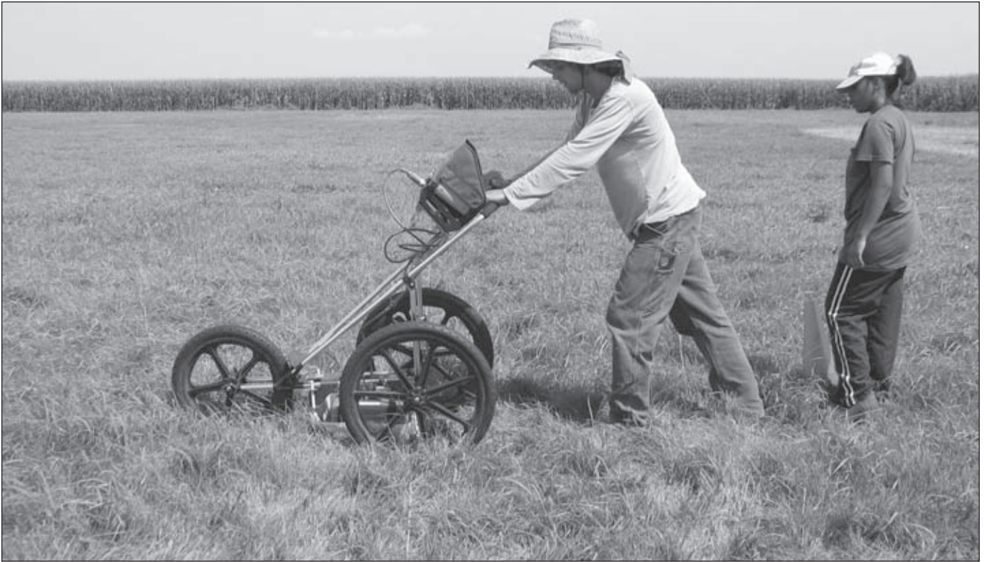
FIGURE 8. Conducting the ground penetrating radar survey with a gpr cart and 400 mHz antenna.
