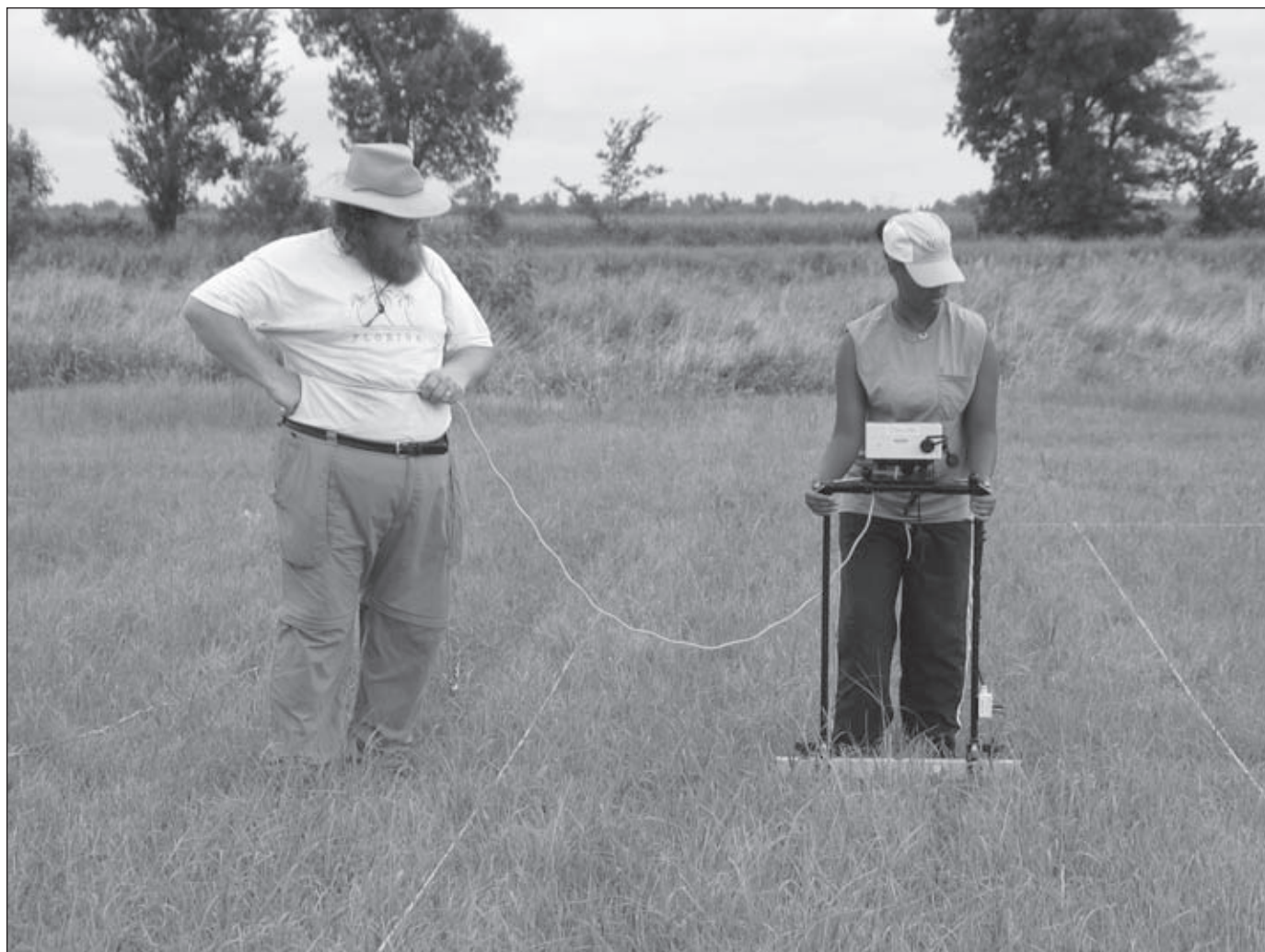
FIGURE 7. Conducting the resistance survey with the resistance meter and twin probe array.
