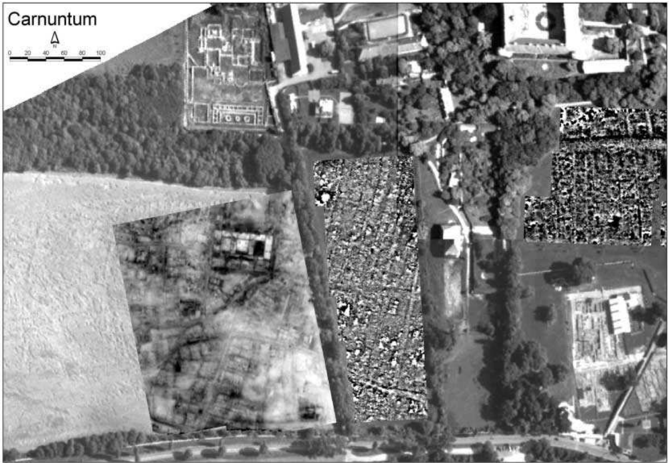
Fig. 5 Aerial photograph (Freigabenr. 13088/15-1.4-99) of the civil town of the Roman Carnuntum combined with the digital image representations of the resistivity mapping ( left ) and the magnetic surveys ( right ) outlining the town's layout. The large building complex visible in the resistivity mapping could be identified as to be the southern part of the forum sought for over 100 years and discovered by prospection in 1996. The monumental buildings are facing to the open square of the forum. The already excavated monumental bath visible in the aerial photograph is situated north of the forum
