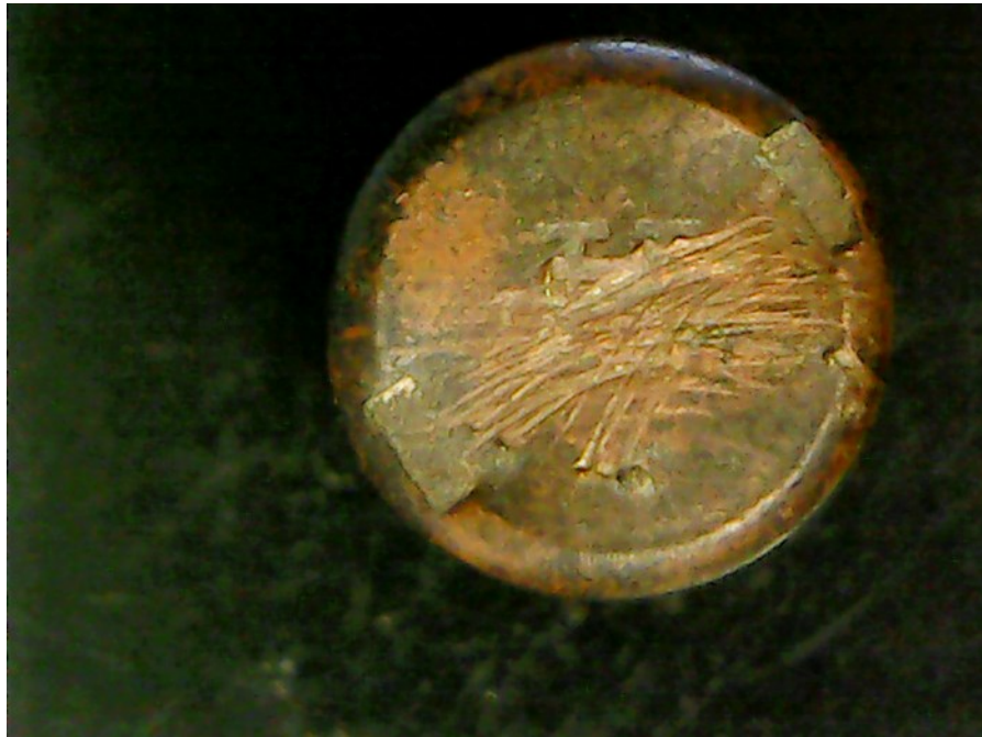
Figure 5. Rectangular firing imprints left on a .22 caliber cartridge by a Sub-Caliber Adapter for a 1903 Springfield Gallery Rifle; note the scratch marks on the cartridge head.
