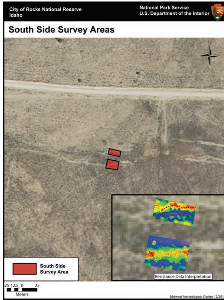
Figure 23. South Side Survey Area map with resistance data interpretation overlay.
