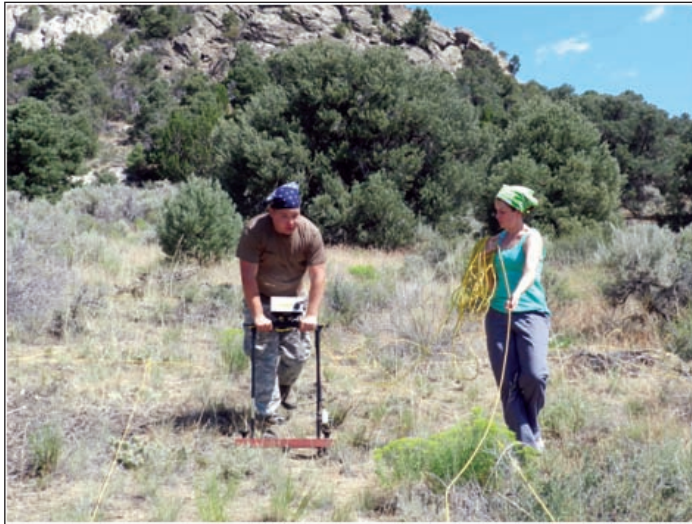
Figure 12. Archeological Technicians Curtis Sedlacek and Ashley Barnett conducting resistance survey (using a Geoscan Research RM15 resistance meter with PA5 multiprobe array) at Pinnacle Pass Survey Area (looking north).
