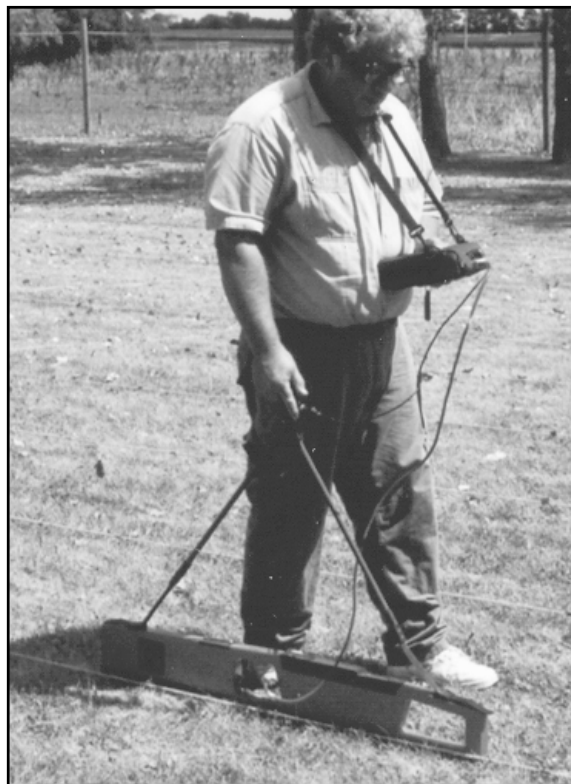
Figure 27. Geonics EM38 ground conductivity meter.
