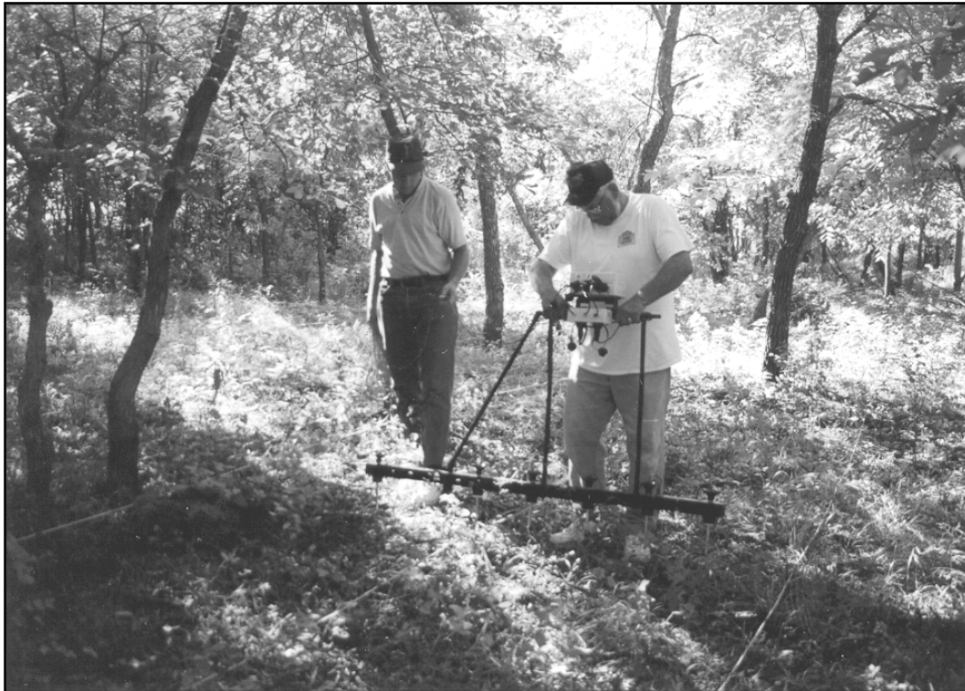
Figure 26. Soil resistance survey with Geoscan Research RM15 resistance meter, PA5 multiprobe array, and MPX15 multiplexer; view to the south.
