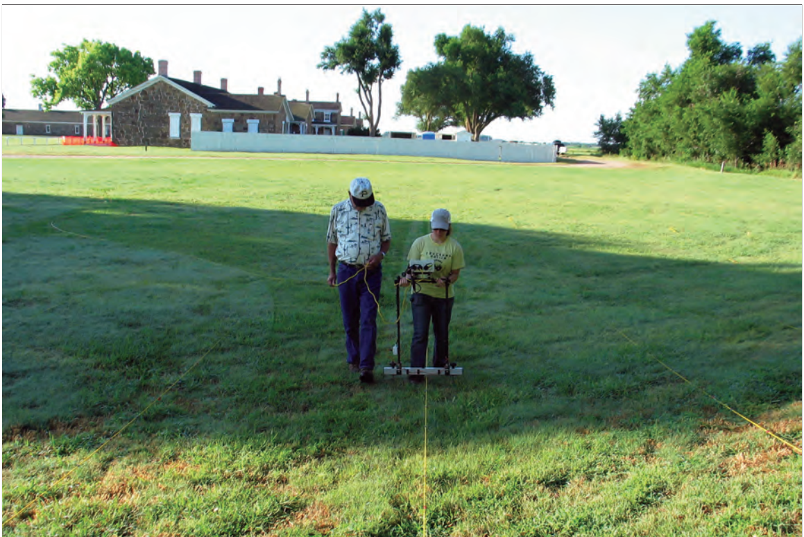
Figure 10. Conducting the resistance survey with the resistance meter and twin probe array (view to the south southeast).
