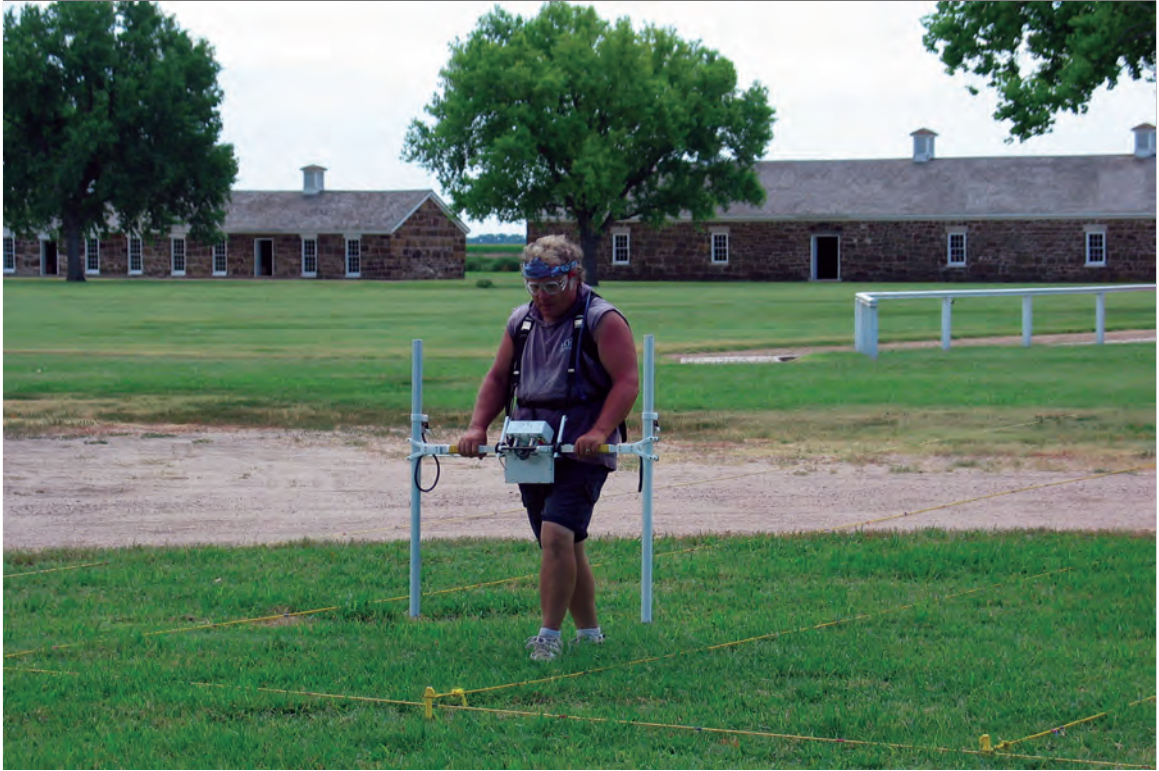
Figure 9. Conducting the magnetic survey with the dual fluxgate gradiometer (view to the southeast).
